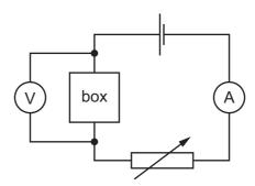
The variable resistor is adjusted and measurements are taken to determine the I-V characteristic for the box, as shown.
