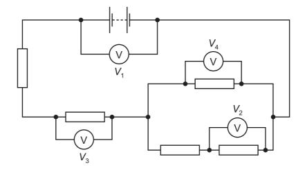
The reading  $V_1$  is 8.0 V and the reading  $V_2$  is 1.0 V.
